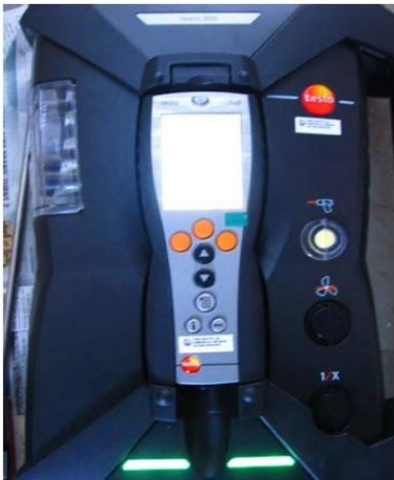
Figure 16: Flue gas analyzer for analysis of air pollutants
