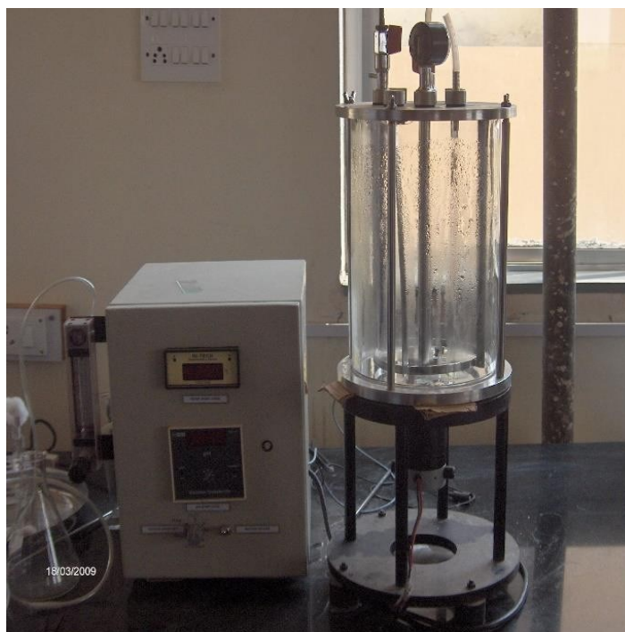
Figure 5: Performance Liquid Chromatography system for analysis of biological metabolites Figure 6: FERMENTER for lab scale production of industrially important compounds
