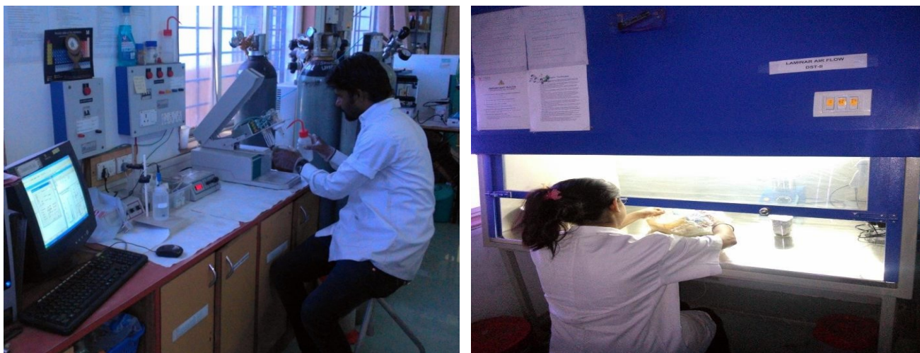
Fig. 2 - Laminar hoods for sterile work space
