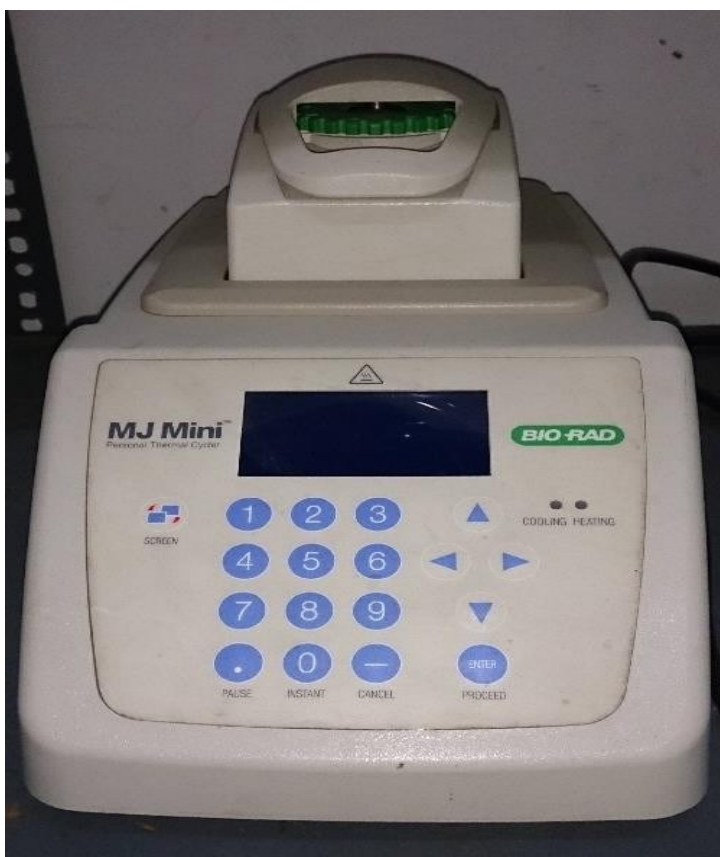
Figure 9: Thermocyclers and Gradient PCR for molecular and nucleotide research
